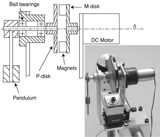
Fig. 1. Sketch and photograph of the experimental setup. The pendulum rotates about the axis  $\Delta$ . The coupling between the pendulum and the motor is due to magnetic forces (there is no contact) between the aluminum disk (P-disk) attached to the pendulum and the disk with the magnets (M-disk) attached to the rotor of the motor.
