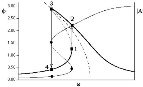
**Fig. 5.** The hysteresis in the response diagram for  $\beta < 0$ . The jump occurs from point 1 to 2 when the driving frequency increases and from point 3 to 4 when the frequency decreases. The dashed line represents free oscillations. With the dotted line we marked the non-physical solution.
